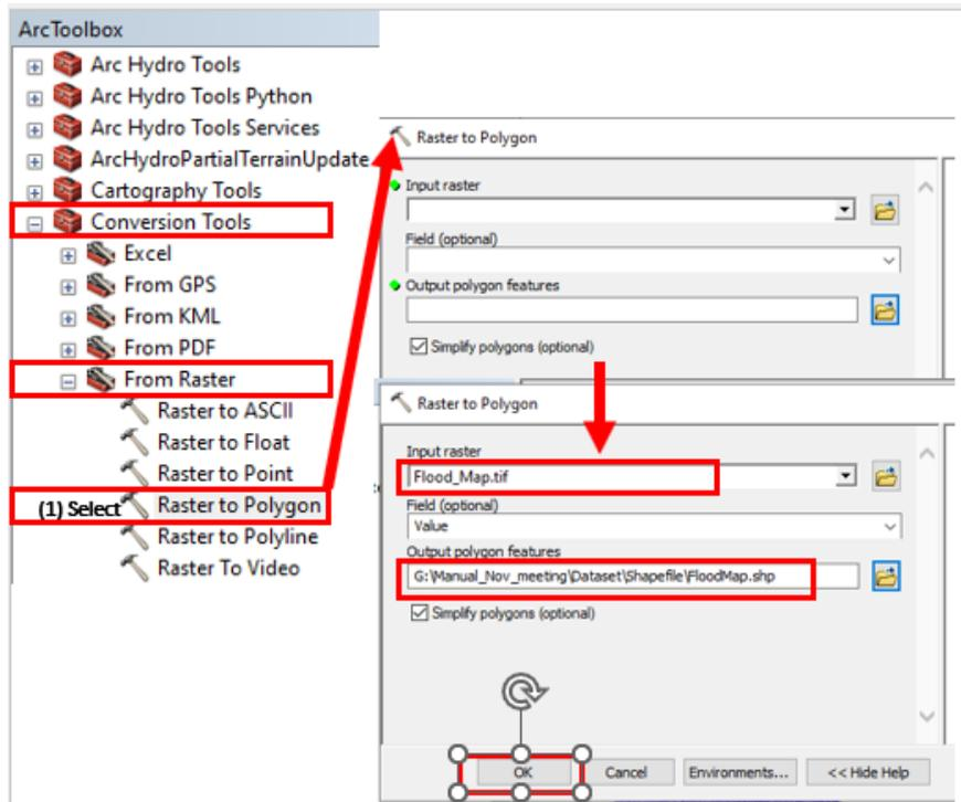
Figure C-100 Convert flood layer to shapefile
