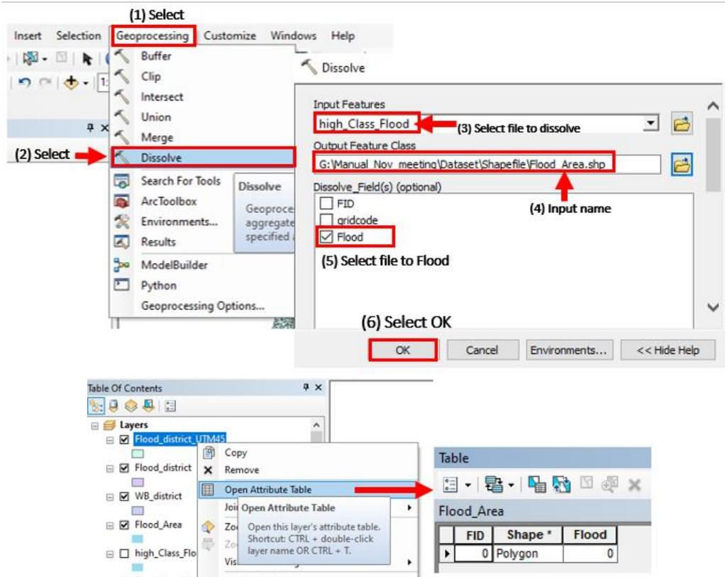
**Figure C-105 Dissolving shapefile with high and very high flood classes into a single flood area**
