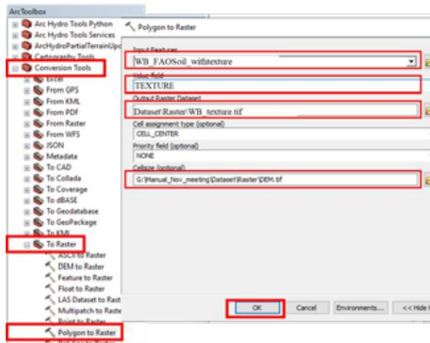
Figure C-50 Convert soil shapefile to raster based on soil texture
