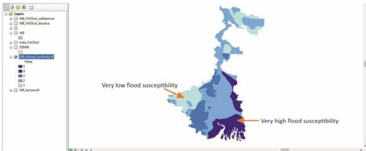
**Figure C-52** Output result of reclassified soil layer with colour scheme
