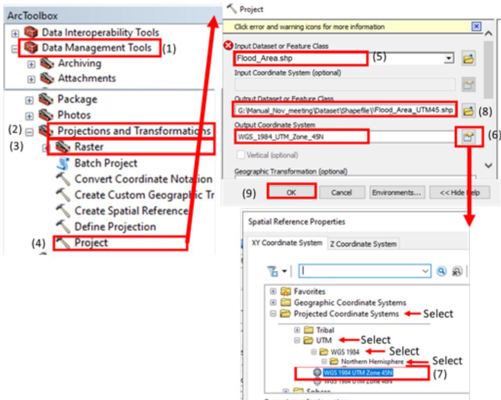
**Figure C-107 Projecting flood shapefile to UTM Coordinate System**
