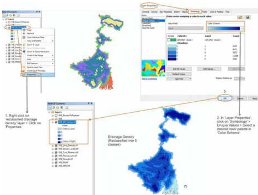
**Figure C-13 Assign a colour scheme to the reclassified drainage density layer**
