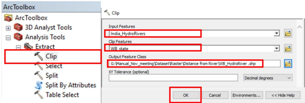
**Figure C-9 Clip Hydrosched Rivers network shapefile for AOI**
