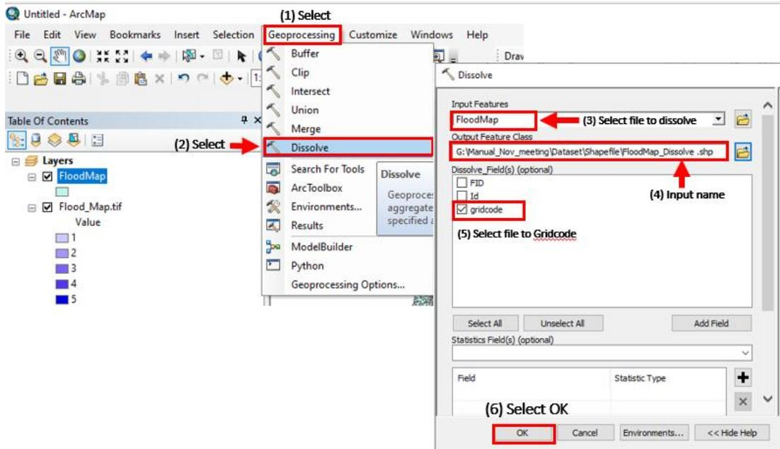
**Figure C-101 Dissolve polygon feature in the flood layer**
