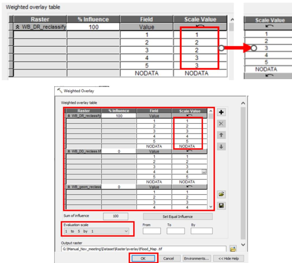
Figure C-98 Insert evaluation scale for weighted overlay
