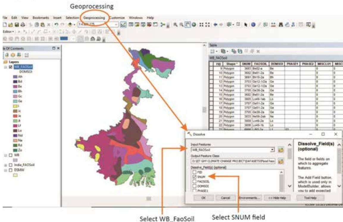
Figure C-42 Dissolve soil layer based on SNUM classes
