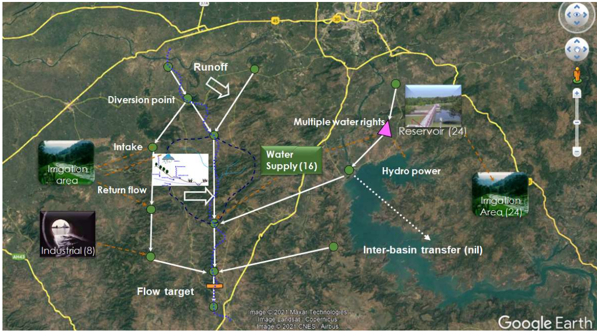
Figure 55: Operation of Rani Avanti Bai Sagar irrigation project
