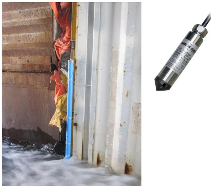
**Figure 4** A pressure probe in a tube, mounted at the same sampling site as the ultrasonic water level sensor in Figure 47 and an example of a pressure probe (www.nexsens.com)
