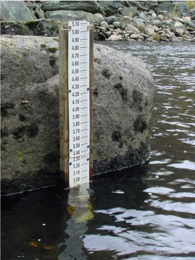
Figure Example of a record site with a staff gauge (Crawford, 2012)
