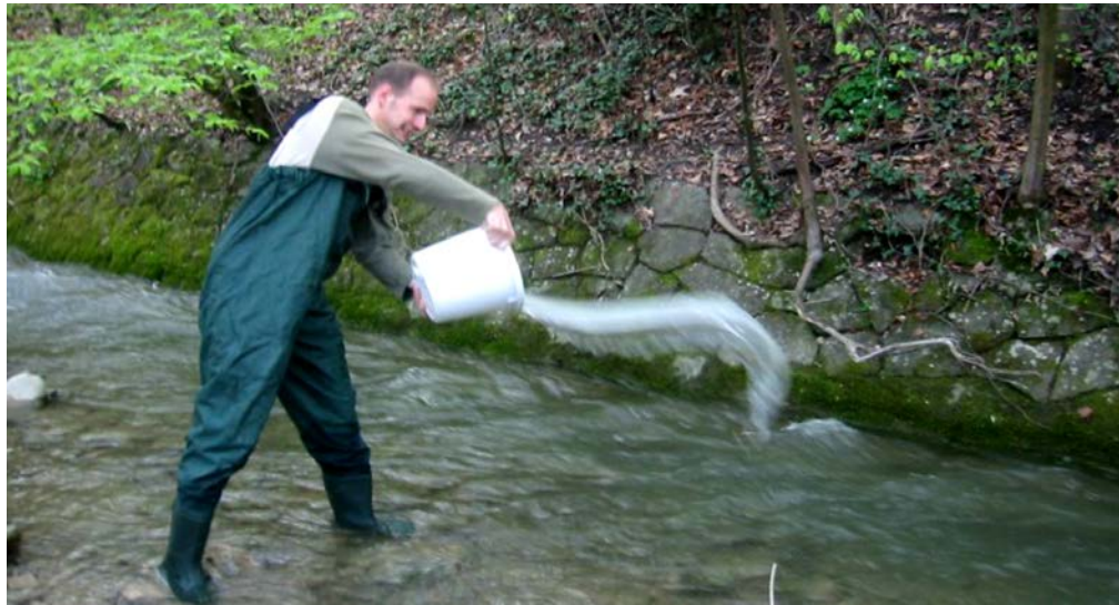
Figure The dissolved salt is injected momentarily by a student (Braun, 2009)
