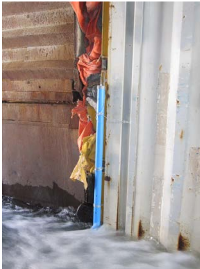
Figure 4 A pressure probe in a tube, mounted at the same sampling site as the ultrasonic water level sensor in Figure 47 and an example of a pressure probe ( www.nexsens.com )
