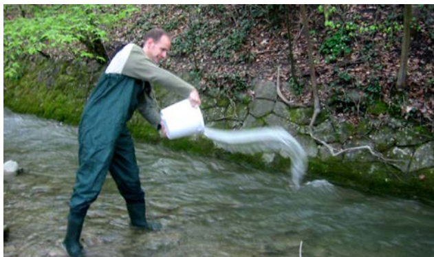
Figure 10 The dissolved salt is injected momentarily by a student (Braun, 2009)
