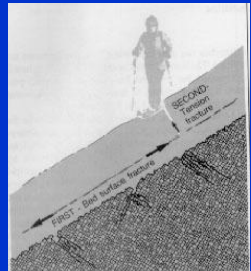
Initial shear fracture produces a crown tension fracture near a skier
