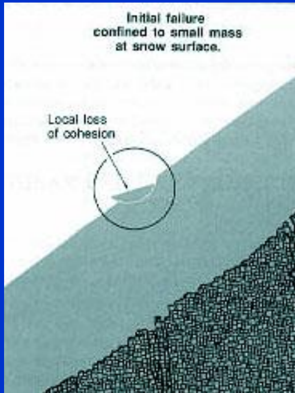
Mechanism of loose snow avalanche failure
