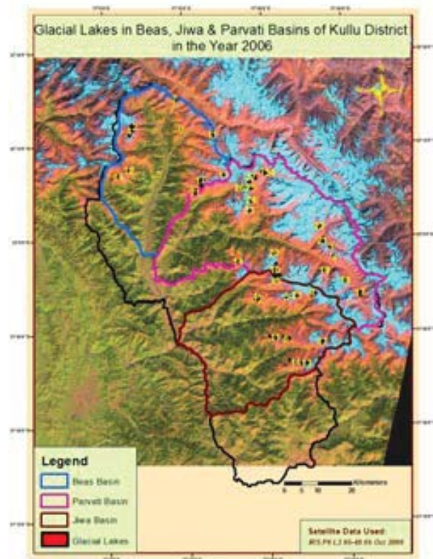
Figure 7: Example of a manually digitized glacier lake inventory compiled for the main basins of the Kullu district using satellite imagery from 2006.
