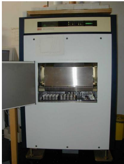
Fig : Ultra Low Level Liquid Scintillation Spectrometer (Front view, internal structure and typical ^3\text{H} & ^{14}\text{C} spectrum)
