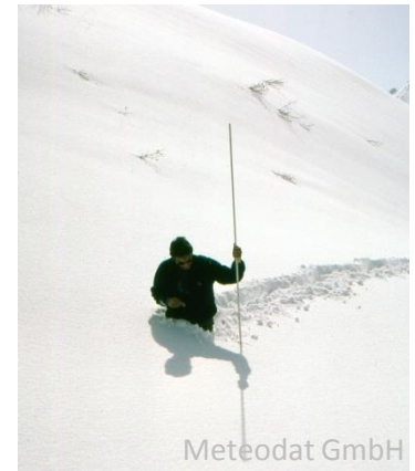
measuring snow depth with a GPS and a snow probe
