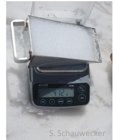
Weighting the snow probe with a digital balance
