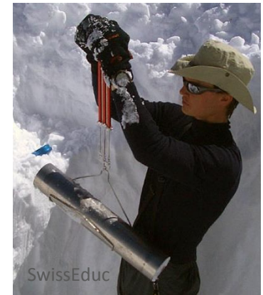
Weighting the snow probe with a spring balance
