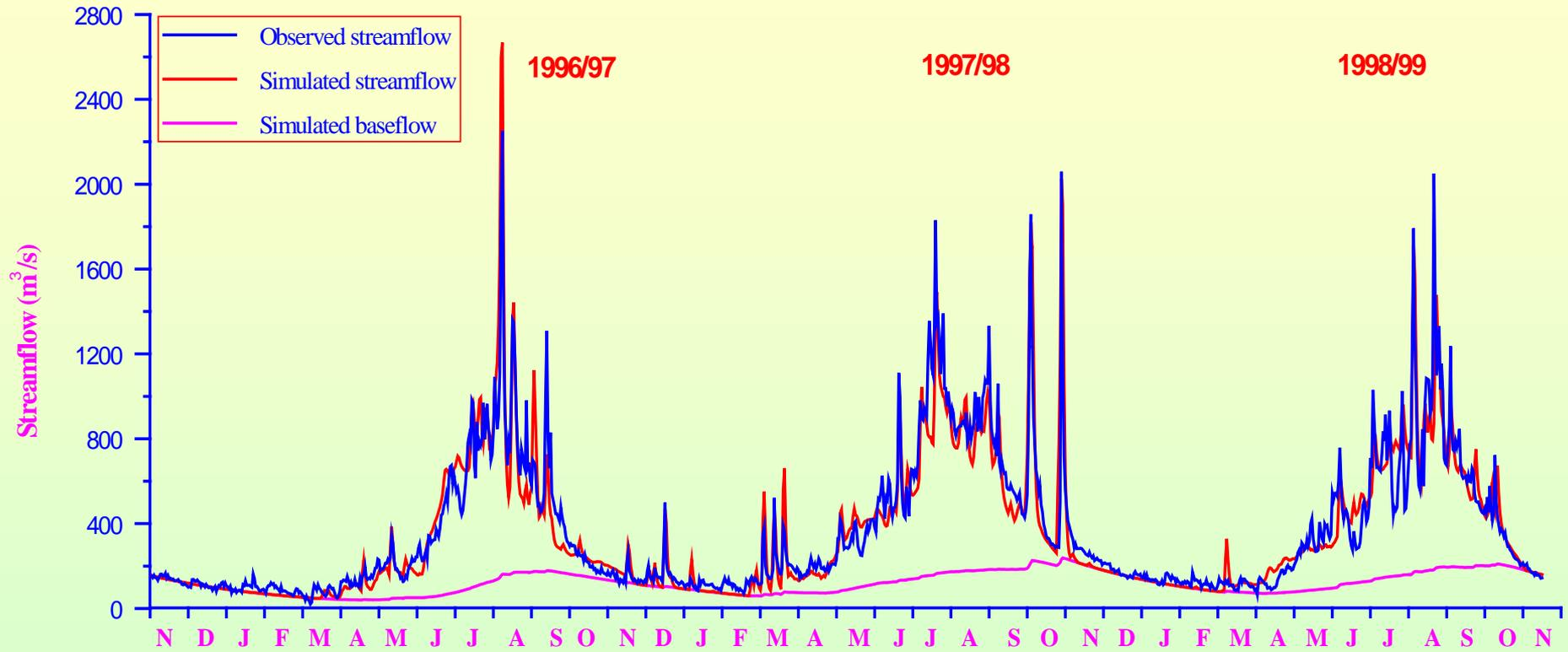
Figure 4: Observed and simulated daily streamflow for the Satluj River at Bhakra for a period of 3 years (1996/97 - 1998/99).
