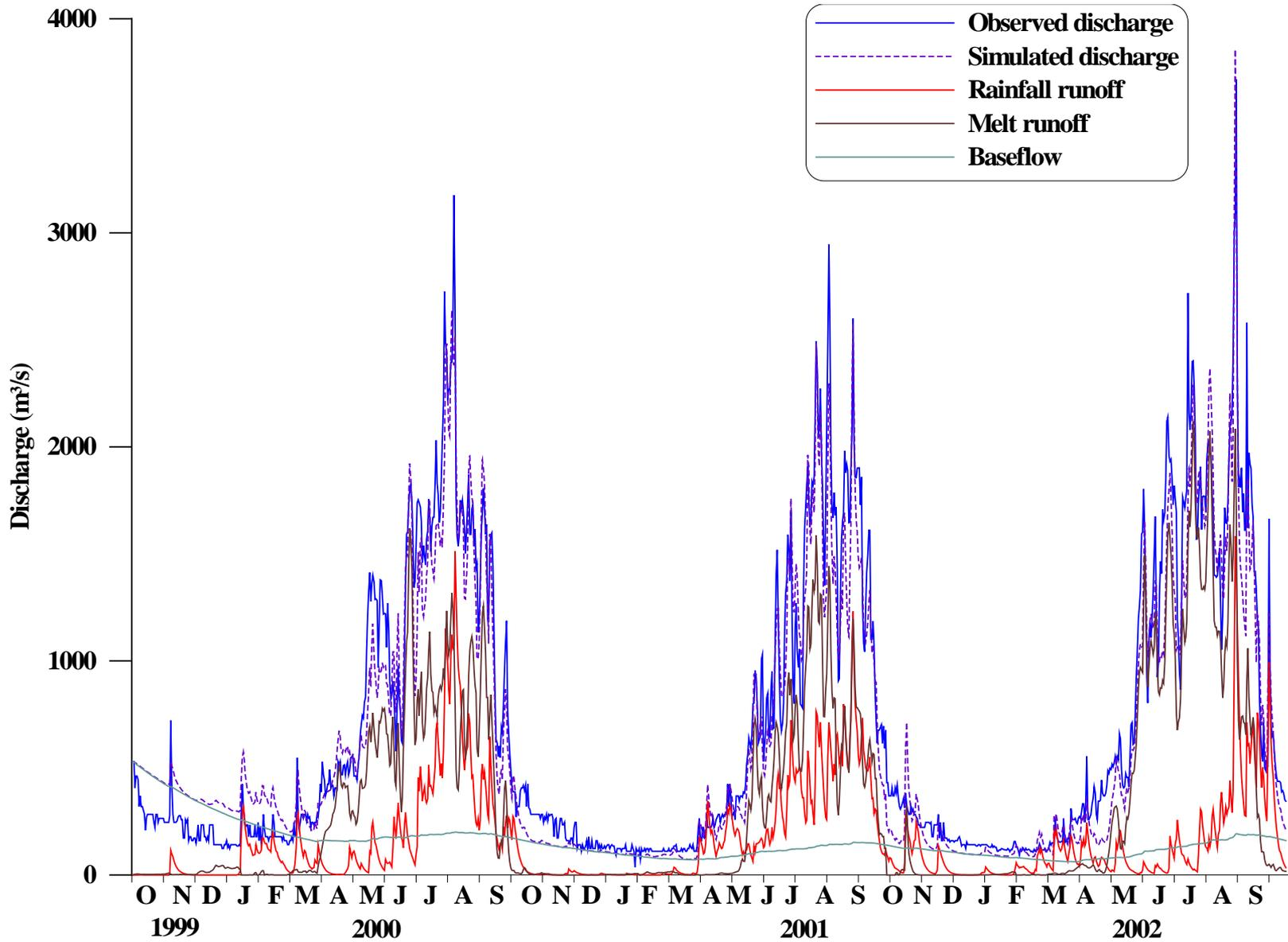
**A comparison of observed and simulated discharge of the Chenab River at Salal Dam for the simulation period (1999/2000 to 2001/2002).**
