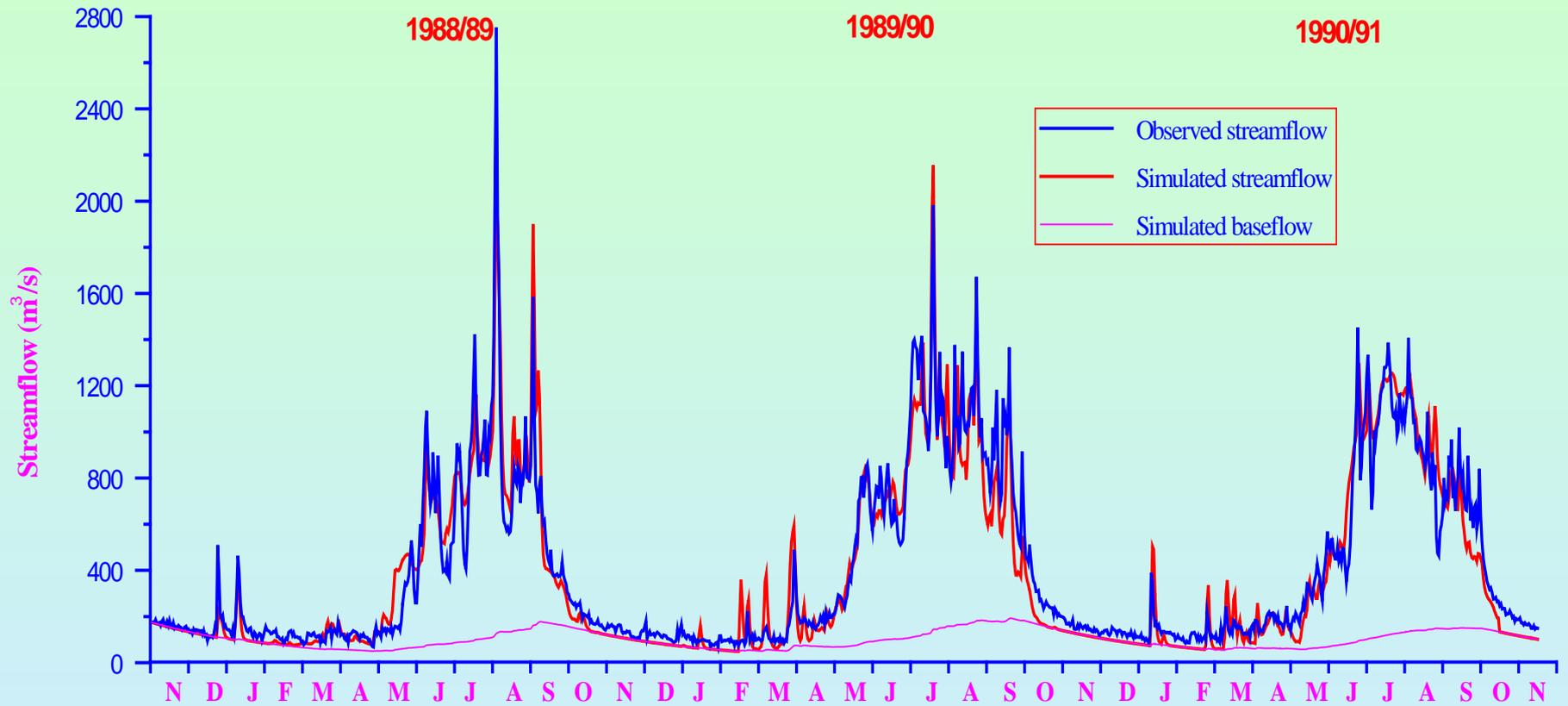
Figure 1: Observed and simulated daily streamflow for the Satluj river at Bhakra for a period of 3 years (1988/89 - 1990/91)
