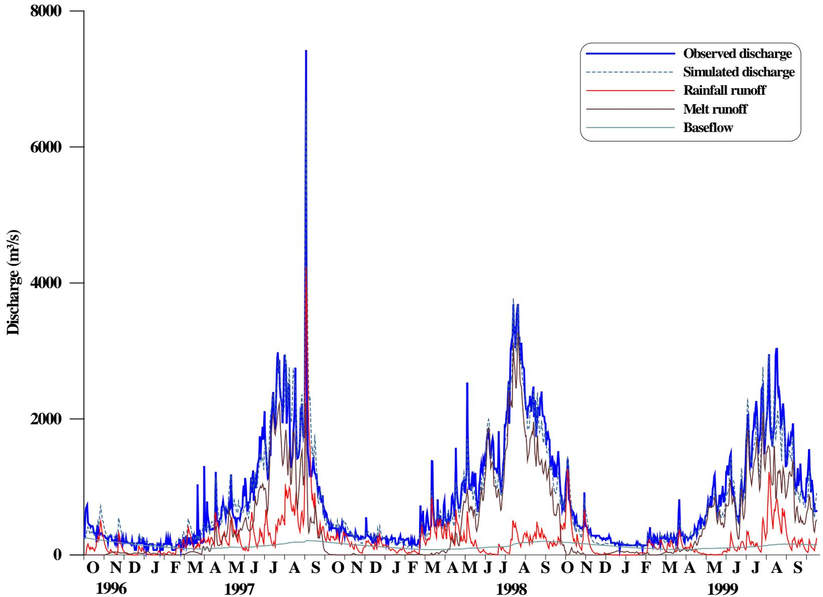
A comparison of observed and simulated discharge of the Chenab River at Salal Dam for the calibration period (1996/1997 to 1998/1999).
