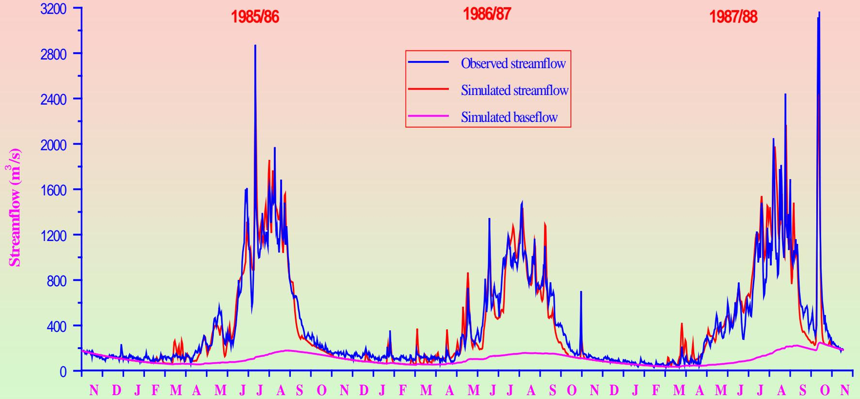
Figure 1: Observed and simulated daily streamflow for the Satluj River at Bhakra for a period of 3 years (1985/86 - 1987/88)
