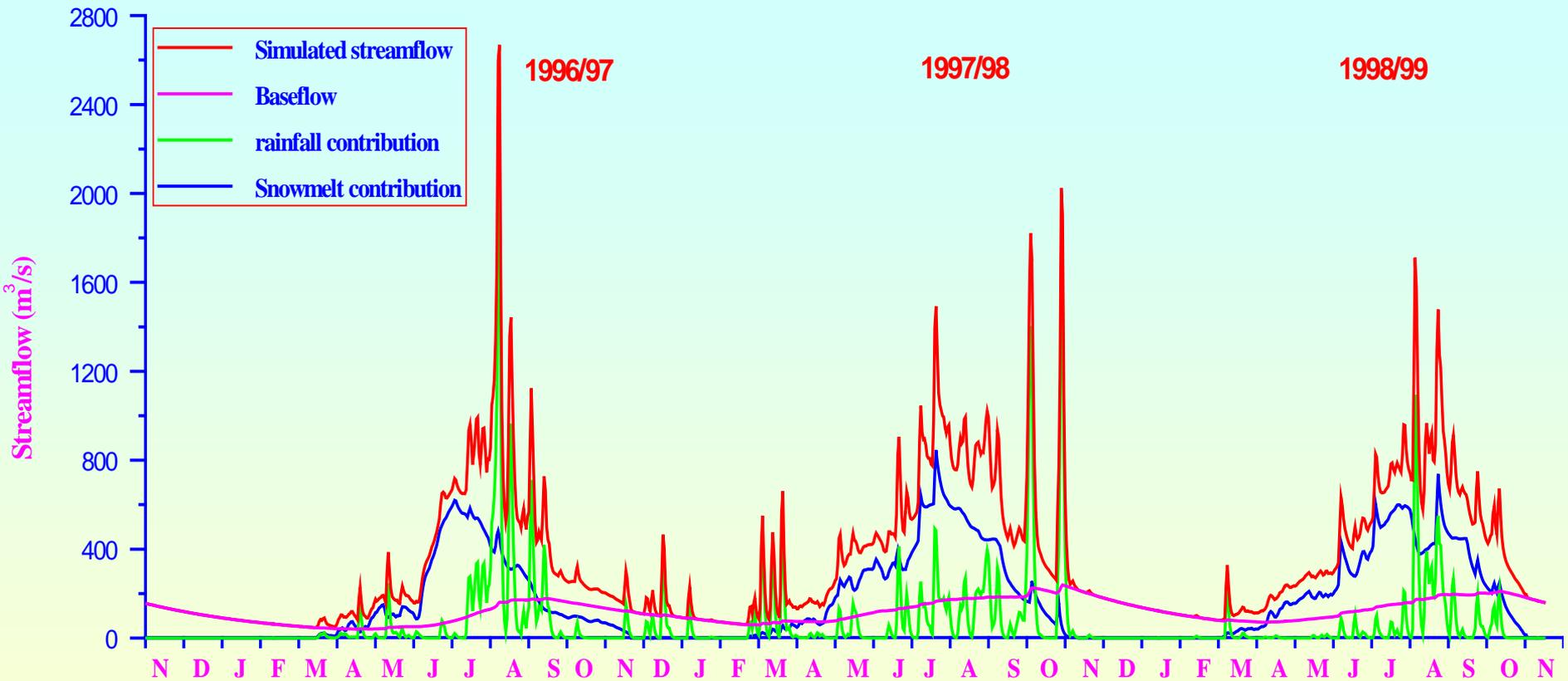
Figure 5: Different components of simulated daily streamflow for the Satluj River at Bhakra for a period of 3 years (1996/97 - 1998/99).
